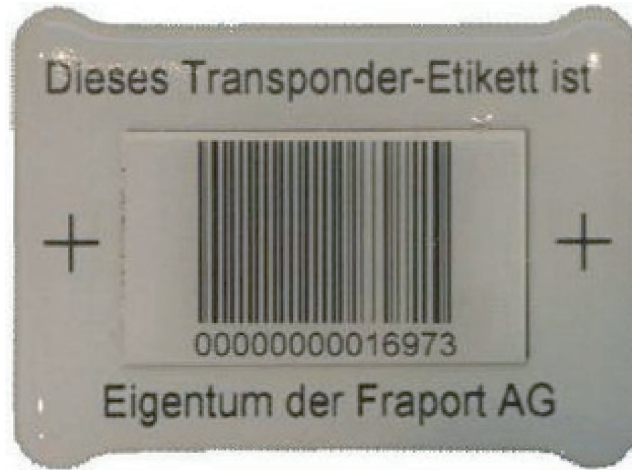
FIGURE 7.3: RFID maintenance tag—also includes a barcode for redundancy
