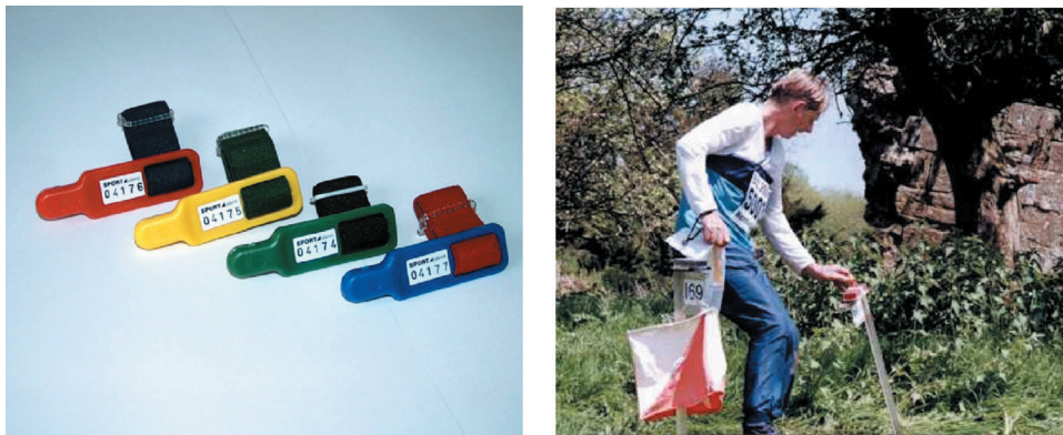
FIGURE 9.2: (a) RFID thumb tags. (b) A control in the forest with RFID writer station and position to insert the thumb tag
