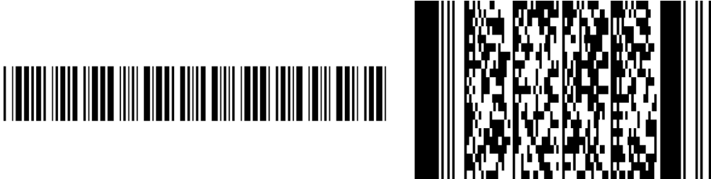
FIGURE 1.1: Examples of (a) 1D (39 Code) and (b) 2D barcodes
