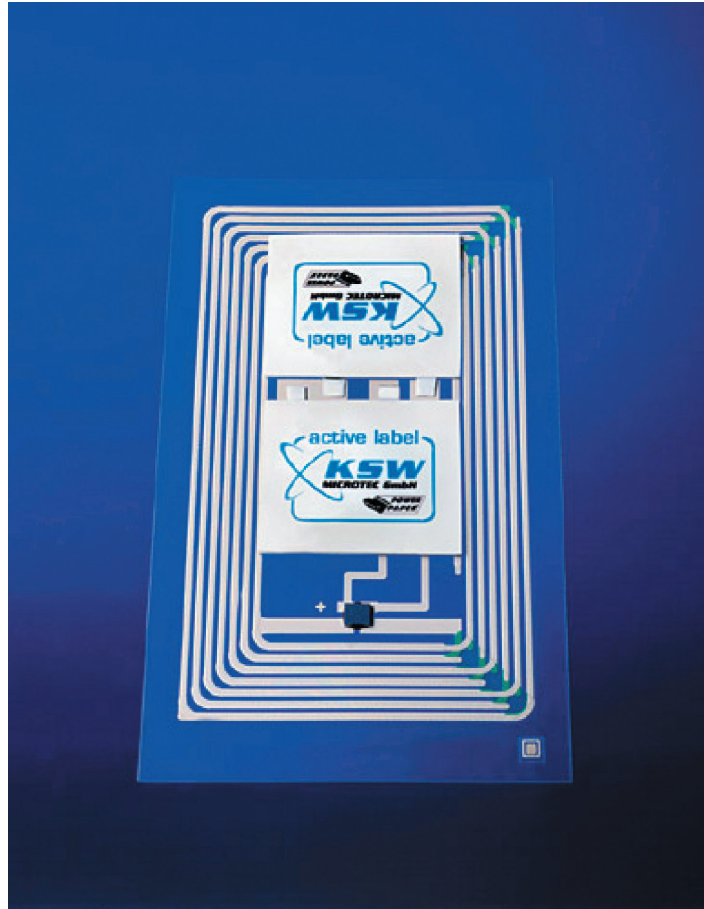
FIGURE 6.1: An RFID tag that can detect a critical temperature threshold (courtesy KSW Microtec AG)
