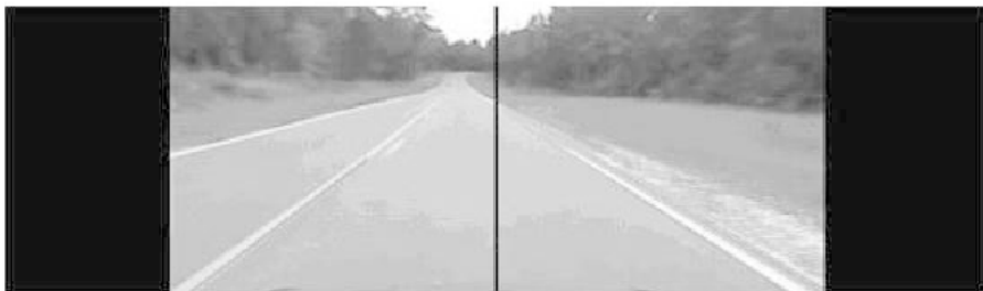
Figure 2.4 Lane lines extracted from the Hough transform. (From: [4].)
