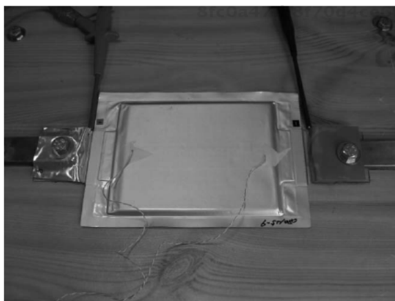
Figure 4.21. Photograph of a 2000 F LIC
