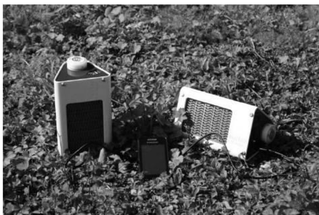
Figure 3.17. Universal USB fuel-cell charger from PaxiTech, fed with a “Hycan” hydrogen can
