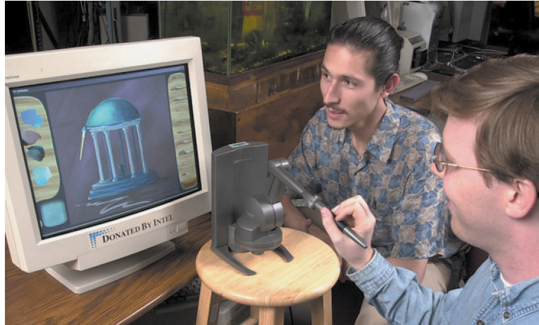
FIGURE 5.4: Haptic painting system setup. An artist using a haptic stylus to paint directly on the virtual canvas using dAb [BSLM01, LBF + 02] (©2002 IEEE).
