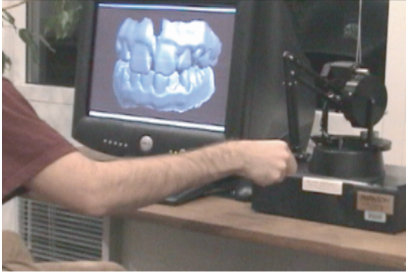
FIGURE 1.1: Example of haptic rendering. A person manipulates a virtual jaw using a haptic device (shown on the right of the image), and the interaction between jaws is displayed both visually and haptically.
