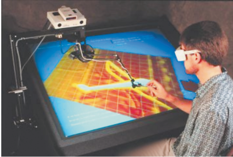
FIGURE 5.2: UNC nanomanipulator system. A virtual reality interface for manipulating nanostructures [TRC + 93, SFL + 06] (©2006 IEEE).
