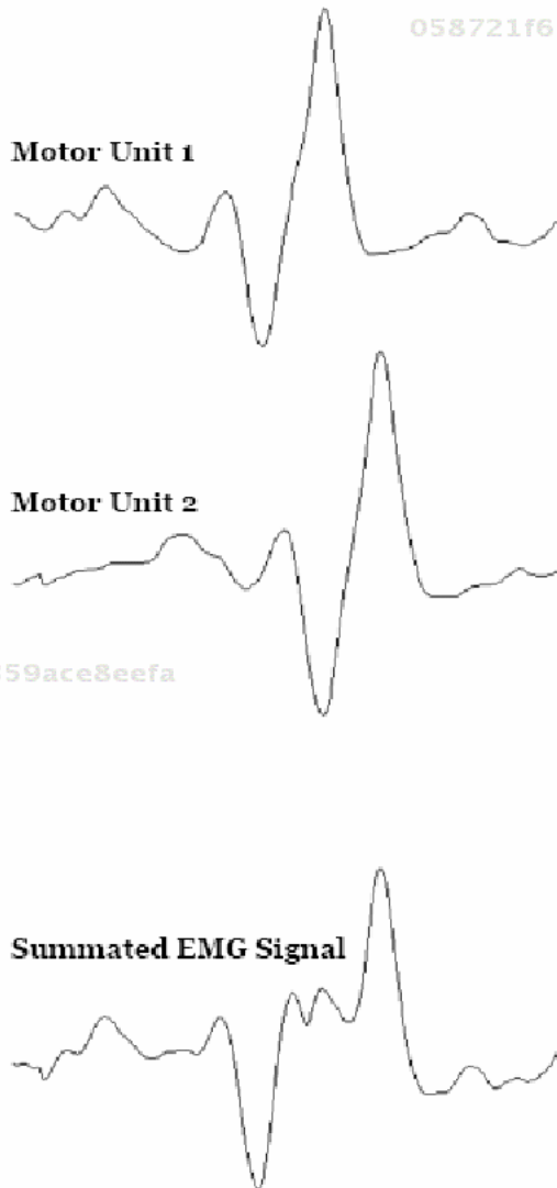
Figure 2. Two simulated motor unit action potentials discharging asynchronously, and the resultant EMG signal representing the sum of these respective motor units.
