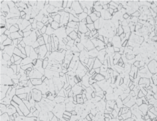
058721f675fce45932afd359ace8eefa Fig. 3.8 Microstructure of 316L plate austenitic phase with grain size ASTM No. 8, hardness 76 HRB. Twinning is observed. Original magnification: 100x. Courtesy of Laboratorios Fairchild S.A.
