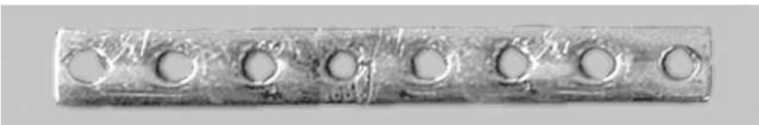
Fig. 9.13 Austenitic stainless steel 316L plate with inadequate mechanical handling
