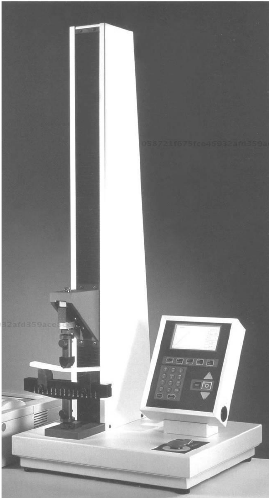
Fig. 5.6 Bend test machine. Bench top Bending Test Machine, Model H5K-S UTM, a 5 kN machine. Courtesy of Tinius Olsen Testing Machine Co., Inc.
