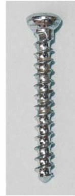
Fig. 3.5 Low-carbon grade 316L austenitic stainless steel cancellous bone screw
