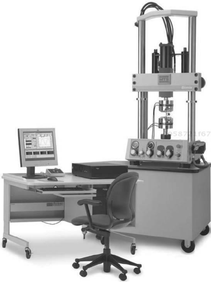
Fig. 5.2 Tension, compression, and fatigue testing machine. The machine shown is an integrated machine, designed to obtain mechanical properties data for both materials and components. © 2009 MTS Systems Corporation. MTS and Bionix are registered trademarks of MTS Systems Corporation. Photo courtesy of MTS Systems Corporation.
