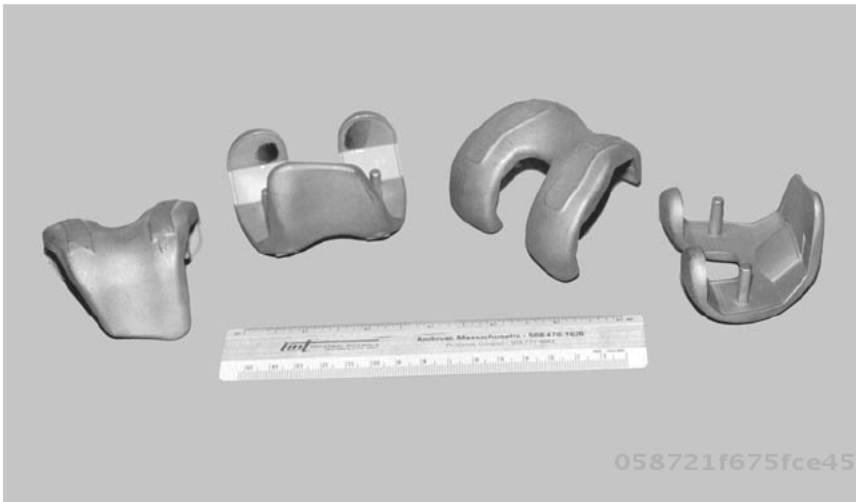
Fig. 3.20 Cobalt-chromium femoral components of total knee joint replacements, made with the hot isostatic pressing (HIP) process, without the final finish. Courtesy of Industrial Materials Technology, Inc.
