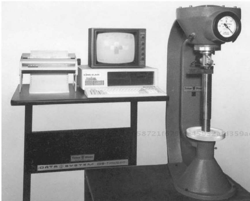
Fig. 5.7 Brinell hardness tester. Tinius Olsen Hardness Tester, with diameter readout system, Model DS/AOB. Courtesy of Tinius Olsen Testing Machine Co., Inc.
