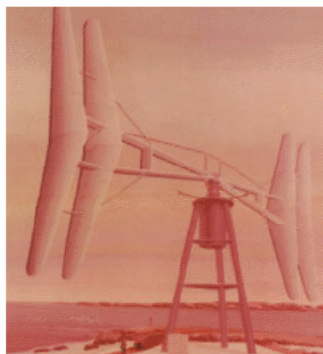
Figure 4.31 Windmill of the big power with blades according to the scheme of a biplane (project).
