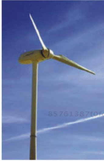
Figure 2.18 AWT turbine behind the basic tower, diameter 26.2 m, power 275 kW at the wind 15.3 m/s, initial wind 5.4 m/s, maximal for the work – 24.6 m/s, hurricane 59 m/s. The tower height - 47.3 m.
