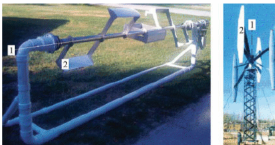
Figure 1.2 Orthogonal high-speed units with the rotation axis (1) perpendicular to the direction of the current. The blades (2) move by the ring routes. Left: a horizontal unit which is effective at invariable directions of the streams (for example, in a mountain valley or on a seashore); right: a vertical wind turbine.
