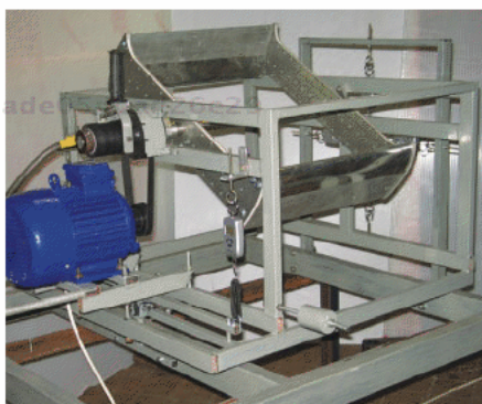
Figure 7.19 The model with electric motor to rotate the blades. In general test the motor did not use. The blades moved by impulse of jets.
