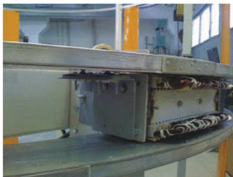
Figure 5.33 The spherical support fixing a gap between the top rotor and the inductor.
