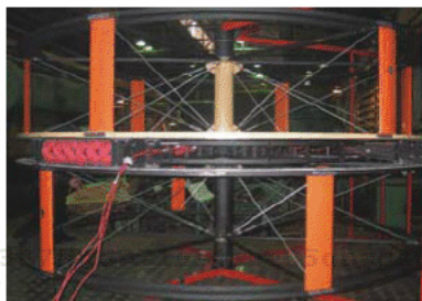
Figure 5.27 Model of the multi-blade unit for the use of the energy of currents. Option for tests in water.
