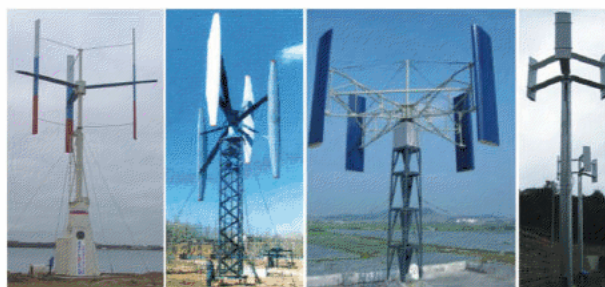
Figure 4.1 At the left windmill NIIES (10 kW), in the center the two-level unit of JSC New Energetic (50 kW), on the right - units of the Chinese firm JOC and JSC Vertical (10 kW).
