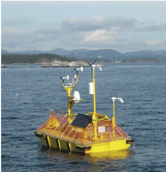
Figure 14-8. The WindSentinel floating lidar system consisting of a Vindicator lidar from Catch the Wind, mounted on a NOMAD buoy developed by AXYS Technologies. Source: AXYS Technologies.
