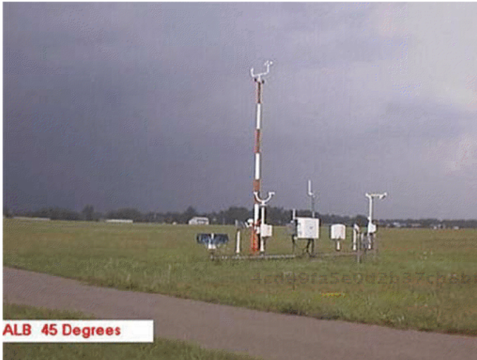
Figure 12-6. The ASOS station at Albany Airport, Albany, New York, USA. Source: National Oceanic and Atmospheric Administration (NOAA).
