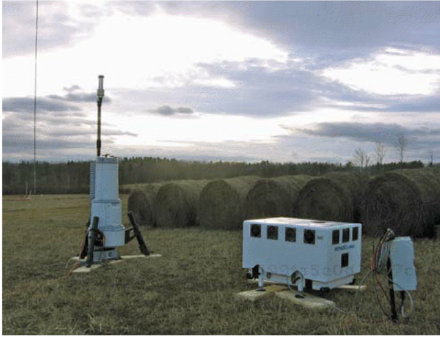
Figure 8-3. NRG/Leosphere's Windcube lidar (left), and Natural Power's ZephIR lidar unit. Source: AWS Truepower.
