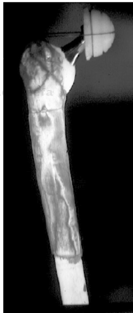
Fig. 9. Photoelastic analysis of an implanted femur.
