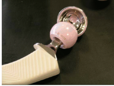
Fig. 10. A ceramic-on-metal hip implant developed at the Institute of Medical and Biological Engineering, University of Leeds 119 .
