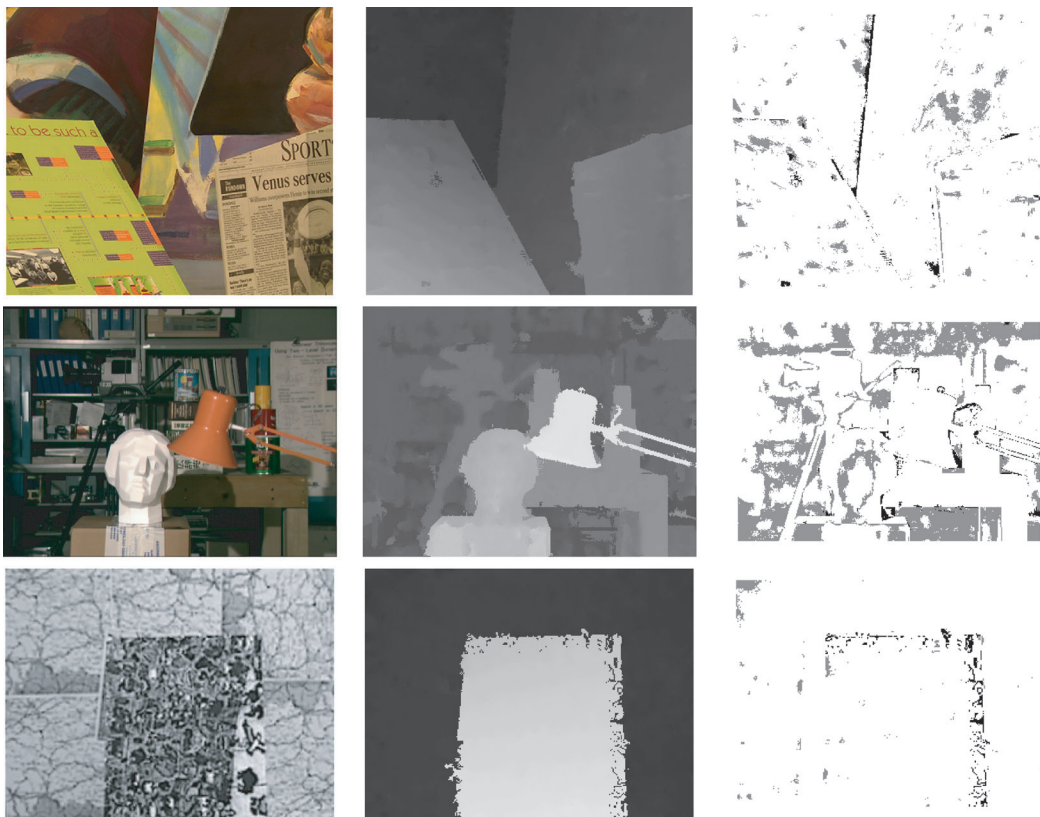
FIGURE 3.7: Left images: final disparity maps and error maps for the “Venus”, “Tsukuba,” and “Map” image pairs from the Middlebury Stereo Evaluation.
