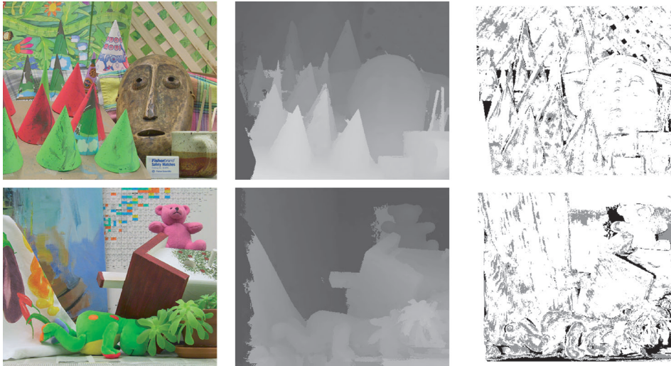
FIGURE 3.8: Left images: final disparity maps and error maps for the “Cones” and “Teddy” image pairs from the Middlebury Stereo Evaluation.
