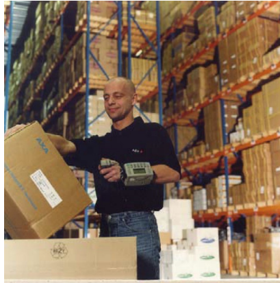
FIGURE 2.2: Symbol’s wrist-mounted wearable computer with ring scanner.
