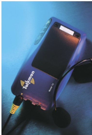
FIGURE 2.11: Vocollect's audio-based wearable computer.
